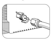
If your antenna ends in a single coaxial lead, simply press or screw the cable onto the antenna terminal on the back of your TV.
